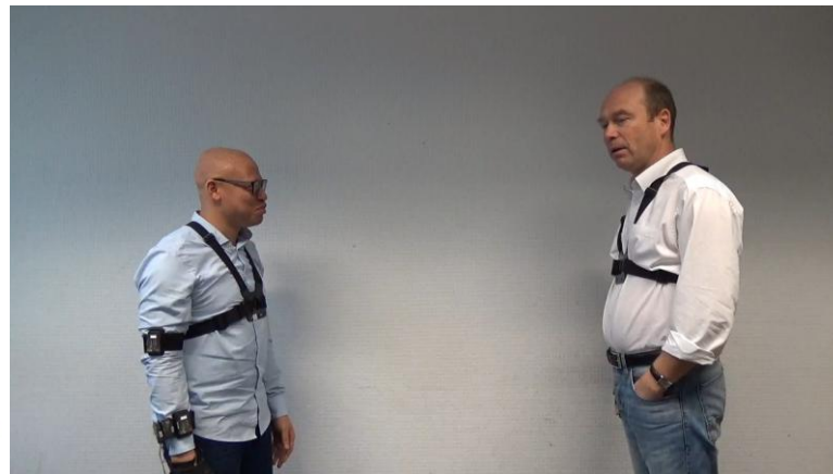
Inertial Measurement Unit (IMU) positions
