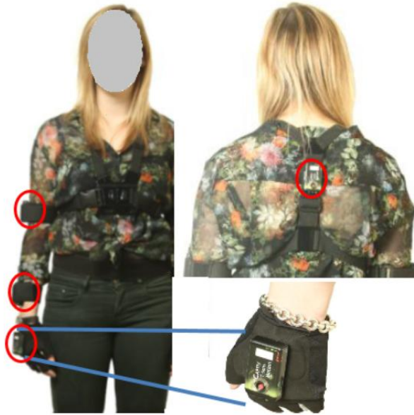
Inertial Measurement Unit (IMU) positions
